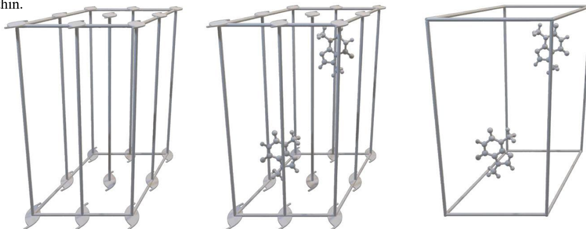
Figure 1. Different visualisations of a unit cell showing only the symmetry elements (left), symmetry elements and molecular content (middle) or only molecular content (right).
